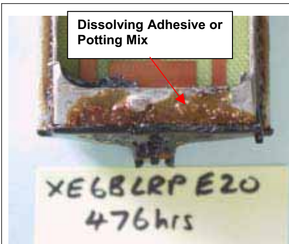
Photograph 3. Fuel sender unit. Close up of adhesive or potting mix being dissolved by E20.
