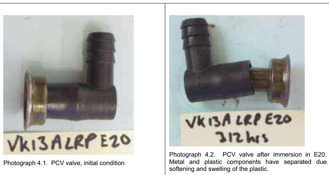
Figure 8.12 PCV Valve Components
