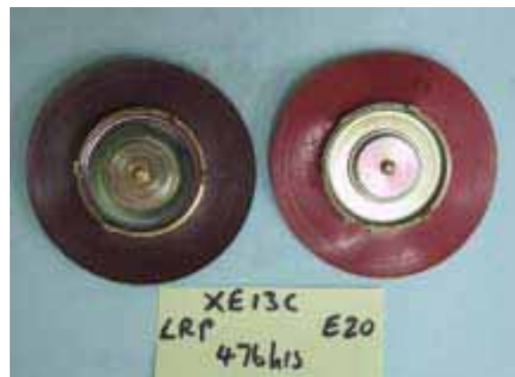
Photograph 4. Fuel pressure regulator diaphragm after immersion in LRP (LHS) and E20 (RHS), showing discoloration in LRP and swelling and distortion in E20.
