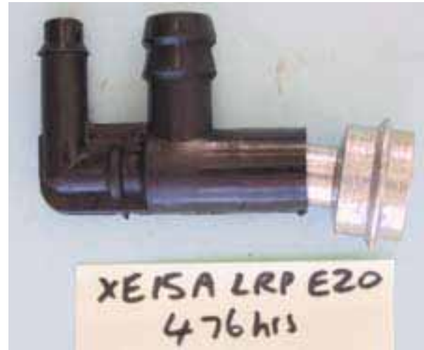
Photograph 2.2. PCV valve after immersion in E20, showing separation of parts due to swelling of the plastic housing.
