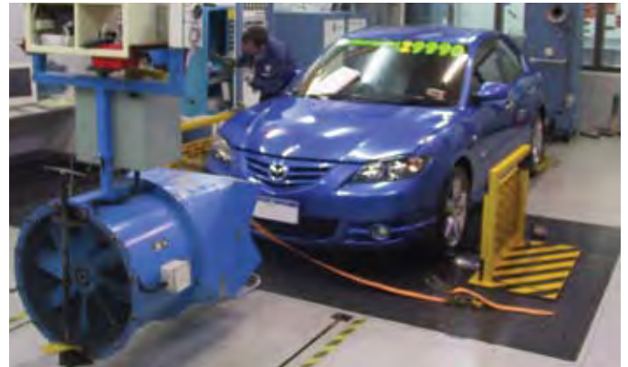
Figure 2: Measuring exhaust emissions—vehicle testing in an emissions chassis dynamometer (ECD) lab.
