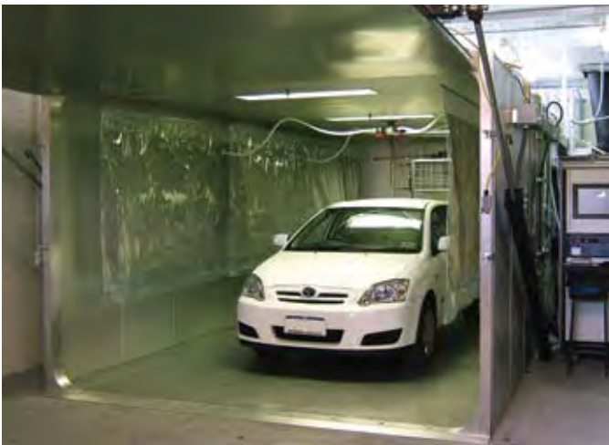
Figure 3: Measuring evaporative emissions—ADR79/01 Variable Temperature Shed.
