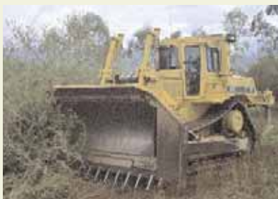
Dozing lantana with a stick rake, Clairview, Queensland (Picture: Mike Richards, courtesy of Queensland Government, Natural Resource Mines and Energy).
