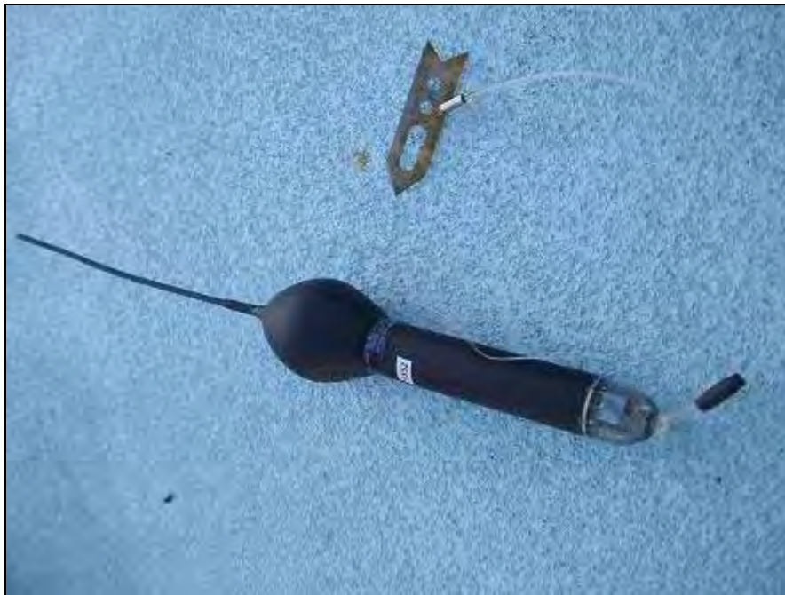
Figure 2.12. PTT-100, Microwave Telemetry Pop-up archival tag showing titanium dart and tether. (Photo - © S. Wilson)
