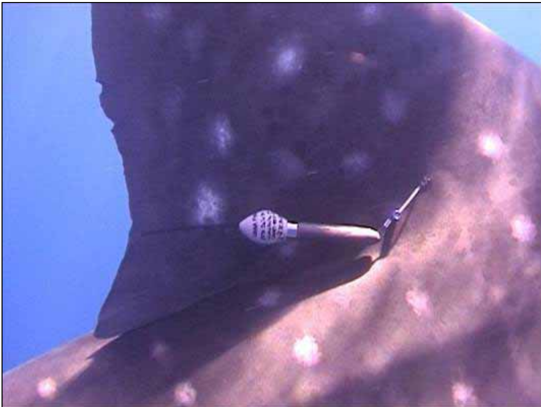
Figure 2.14. PSAT tag embedded in sub-dermal layer of whale shark flank/dorsal fin. (Photo- ©C. McLean)
