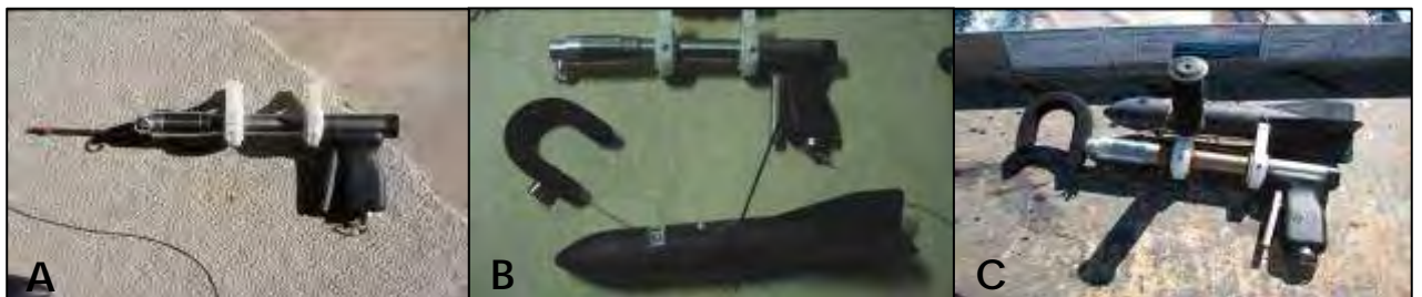
Figure 2.9. A) Applicator & bolt, B) Applicator, fin clasp and satellite tag and C) Satellite tag ready for deployment (Photos A & C © – C. Bradshaw, B © – C. Speed).
