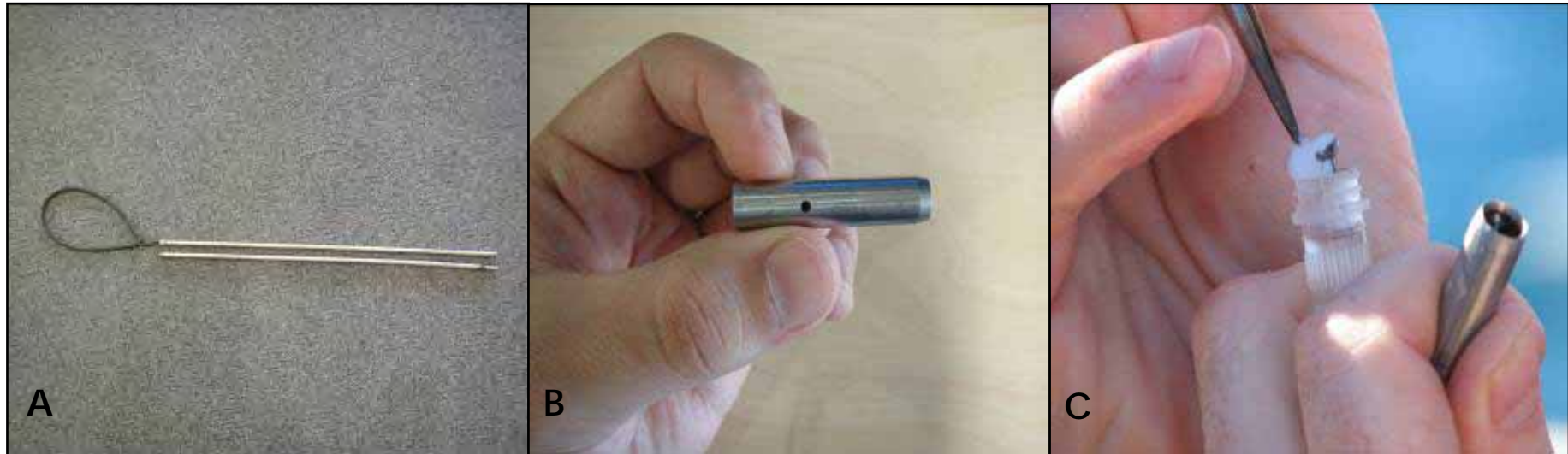
Figure 2.7. A) Hawaiian-Sling pole spear with biopsy tip attached, B) .Biopsy tip for tissue sampling of whale sharks, C) Biopsy tip and whale shark tissue sample being placed in vial of DMSO (Photos A & B – © C. Speed & photo C – © F. Baronie).
