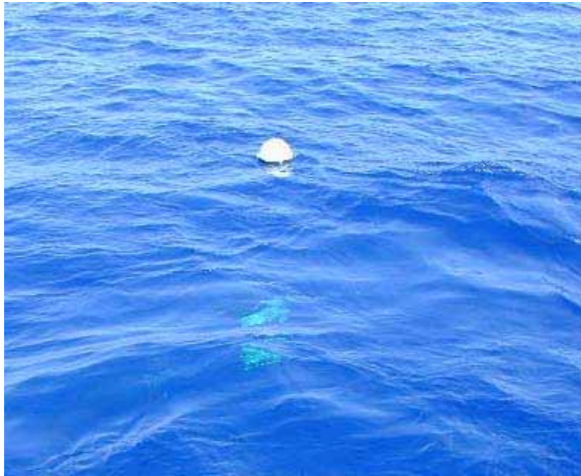
Figure 2: Satellite drifters consist of a floating buoy holding sensor and communication electronics, connected to a sea-anchor. (Reproduced from http://www.aoml.noaa.gov/phod/dac/gdp_drifter.html )
