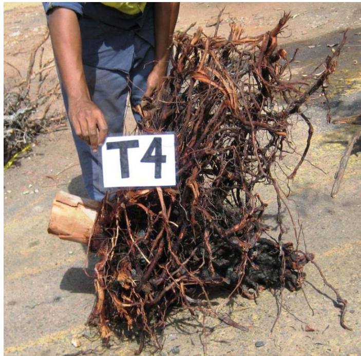
Figure 4 Rootball of 7.7 m high Eucalyptus glomericassis excavated from a trial rehabilitation site on the eastern edge of the Ranger tailings dam (from the so-called, 'Heritage' site). While shallow lateral roots have been broken off, the main primary (tap) root is intact.
