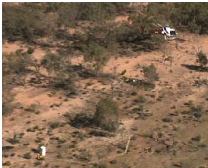
A helicopter trailing the electromagnetic survey receiver over Broken Hill. Data from the survey will be used to help identify available aquifers and possible sites where managed aquifer recharge may be implemented. (DEWHA)
